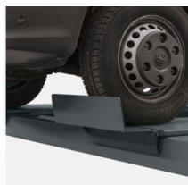
■ The 4 post lift is equipped with a pneumatically unlockable lowering device (every 100 mm). In this way cables and hydraulic system are relieved. Due to the adjustable ratchet strips in the lifting posts, the lift can be aligned in an absolutely horizontal way.
