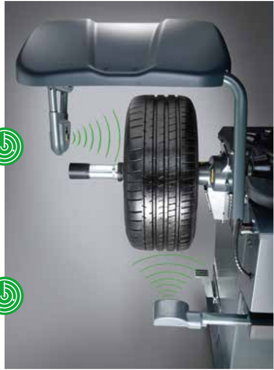
Two sonars measure the number of spokes, wheel data, correct centering and runout
