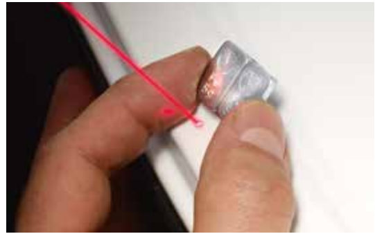
Spot laser* for accurate positioning of adhesive weights on aluminium rims (interior and behind the spokes)
