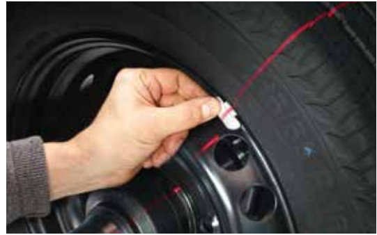
Line laser* for the exact positioning of clip-on weights on the exterior of steel rims
