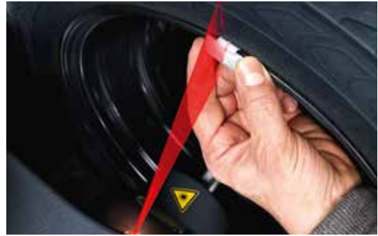
Line laser* for the interior of steel rims
