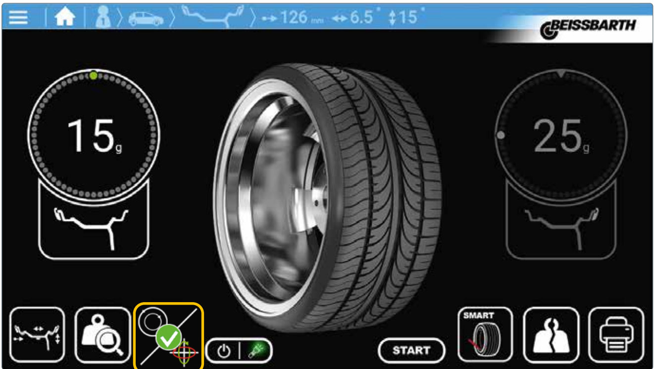
Every wheel gets a radial runout check (eccentricity)
