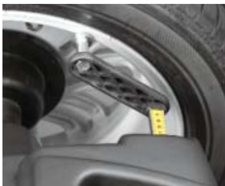
Standard on the MT 835.A: the electronic sensing arm measures wheel rim distance and diameter.
