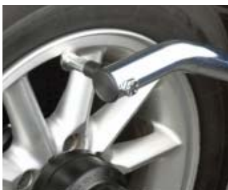
Standard on the MT 835.A: the electronic sensing arm measures wheel rim width.
