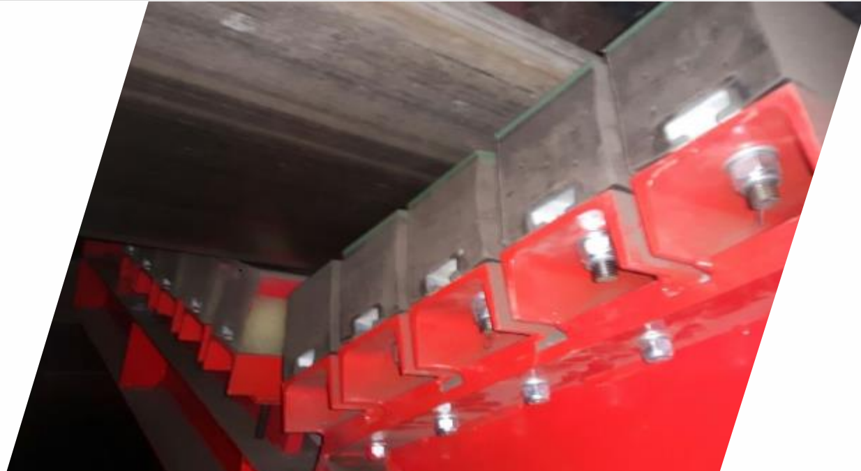
Side view of the impact bars and the impact cradle (manufactured by TIP TOP Borna, subsidiary Nauen)
