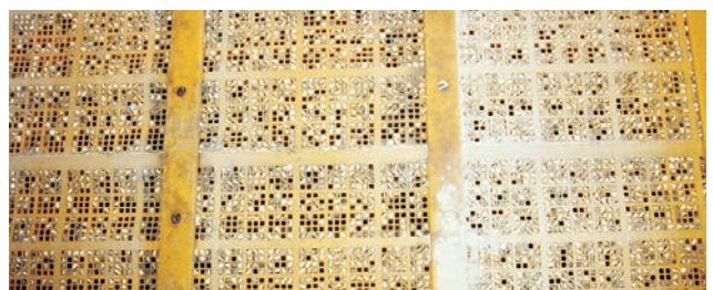
Moulded PUR-screen mats with over 50% pegging material. Efficiency is due to the loss of open screening area, drastically reduced.
