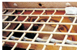
Wear to longitudinal bracings with a steel screen mat.
