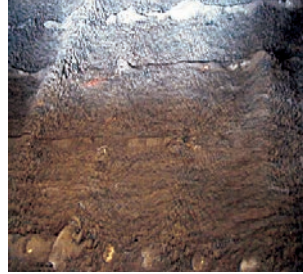
Steel screen mat shows 100% caking.
