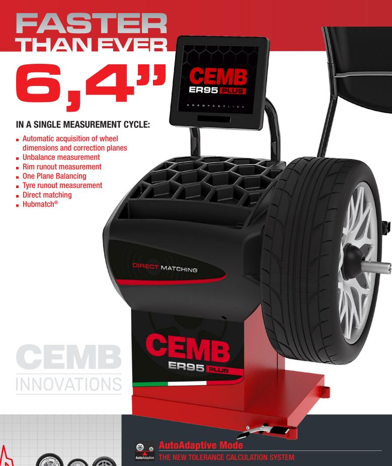
■ The innovative tolerance calculation system **AutoAdaptive Mode** is based on the evaluation of the residual imbalance limit value corresponding to an acceptable perceived vibration. For each wheel that is balanced, the software AutoAdaptive Mode detects weight and dimensions and calculates the tolerance value that will cancel any vibration perceived on the steering wheel. AutoAdaptive Mode grants the highest comfort when driving, and together with **OPB** program, saves balancing time.
